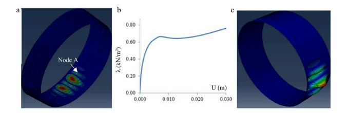
Damage computed for a tank with D = 45 m and H = 12 m. (a) Deflected shape for damage DS1; (b) Equilibrium path for node A (DS1); (c) Deflected shape for damage DS2 (critical mode). Credit: *Emergency Management Science and Technology* (2023). DOI: 10.48130/EMST-2023-0019
