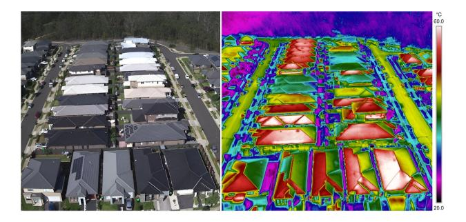
You can clearly see here the difference roof color makes. On the left, you can see the real view of a new housing estate. On the right, an infrared camera shows you the difference in heat (redder = hotter, green = cooler. Credit: Sebastian Pfautsch, <u>CC BY-ND</u>
