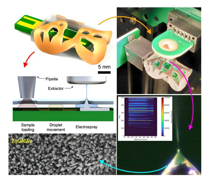
Researchers designed electrospray emitters as externally-fed solid cones with a specific angle that leverages evaporation to strategically restrict the flow of
