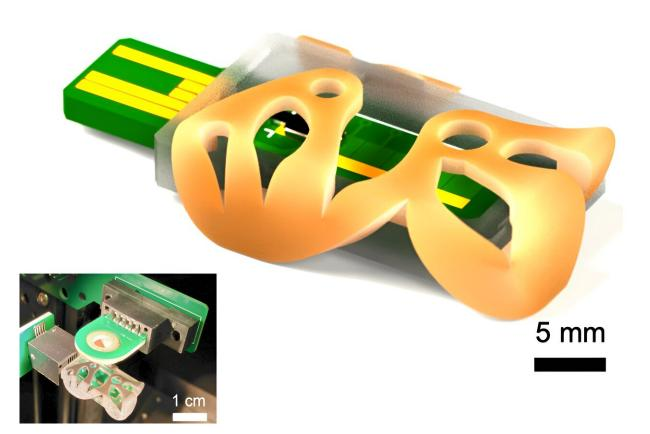
MIT researchers have 3D printed a miniature ionizer, which is a key component of a mass spectrometer. The new miniature ionizer could someday enable an affordable, in-home mass spectrometer for health monitoring. Pictured are parts of the new device, including a green printed circuit board (PCB) with orange casing on top. Under the casing is a black rectangle where the electrospray emitter is located. Credit: Massachusetts Institute of Technology
