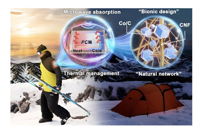
As a result of the bionic design of the neural network-like aerogel-based composite PCMs, both microwave absorption and thermal management are increased, and in colder climates the solar-thermal conversion can be used to heat devices for normal start-up and keep the device closer to an optimal performance temperature. Credit: Beijing Normal University and University of Science and Technology Beijing
