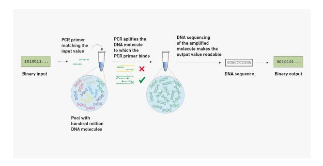
The language of the DNA world uses the letters A, T, C and G. With suitable rules, however, this can easily be translated into a digital sequence of 0s and 1s. Credit: ETH Zurich
