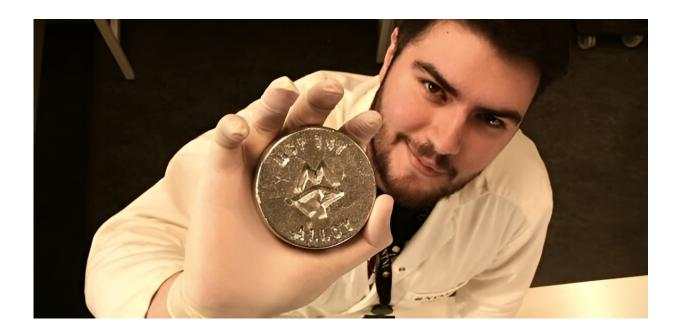
Lewaa Hmadeh, a Ph.D. candidate at NTNU's Department of Geoscience and Petroleum, holds a test well plug made of a bismuth-tin alloy. The marks on the plug show that the alloy is MCP 137, which is made from 58 percent bismuth and 42 percent tin. Credit: Per A.D. Jynge/NTNU
