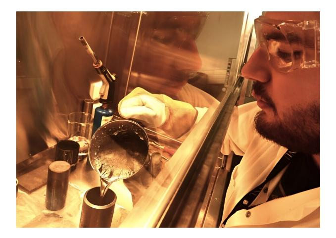
Lewaa Hmadeh in the lab, pouring a molten bismuth-tin alloy inside a steel pipe for his research on well plugs. Credit: Per A.D. Jynge/NTNU
