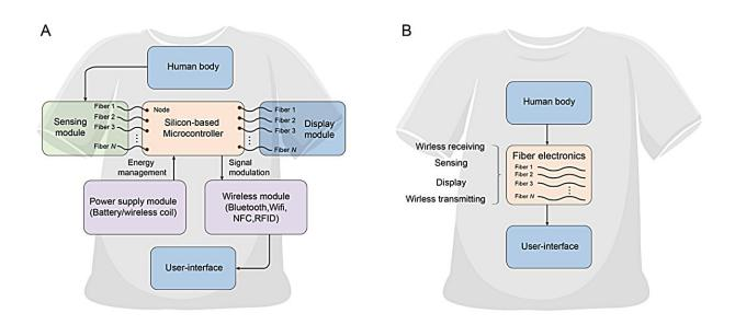
Comparison between (A) conventional chip-based wireless e-textile and (B) chip-based wireless e-textile in this work. Credit: *Science* (2024). DOI: 10.1126/science.adk3755
