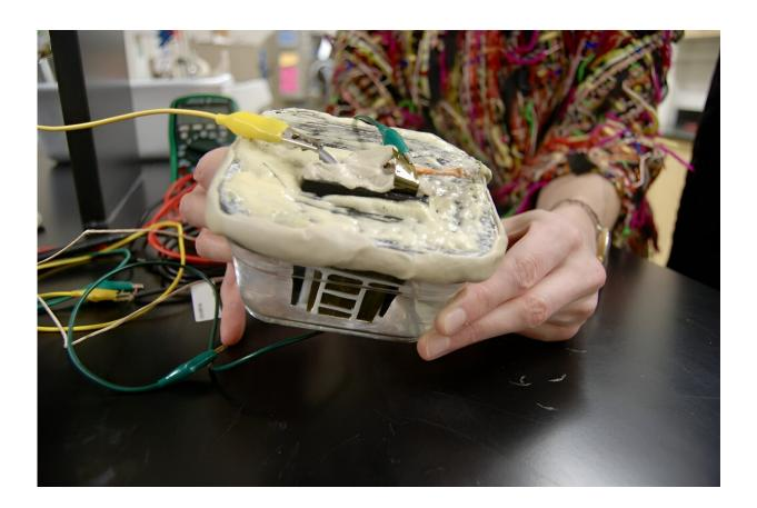
A pyroelectrochemical (PEC) cell, is a device that converts thermal energy into electricity and stores it. Credit: Brian Maffly
