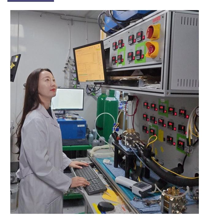
Durability evaluation experiment reflecting solar output variability for green hydrogen production devices. Credit: Korea Institute of Science and Technology
