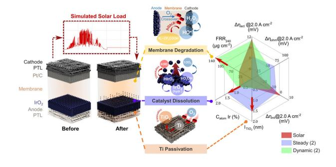
Degradation analysis of key materials for water electrolysis before and after solar-based durability evaluation. Credit: Korea Institute of Science and Technology
