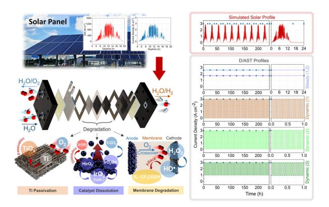
Comparison of solar-based durability evaluation techniques with constant current and cyclic current methods. Credit: Korea Institute of Science and Technology
