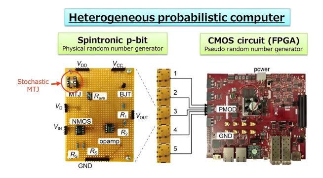
A photograph of the developed prototype. The system is designed such that the spintronic probabilistic bit comprising a stochastic magnetic tunnel junction (MTJ) [left] generates a physical random number that drives the pseudo random number generators programmed in the CMOS circuit, or the field-programmable gate array (FPGA) [right]. Credit: Shunsuke Fukami and Kerem Camsari, adapted from *Nature Communications* (2024). DOI: 10.1038/s41467-024-46645-6
