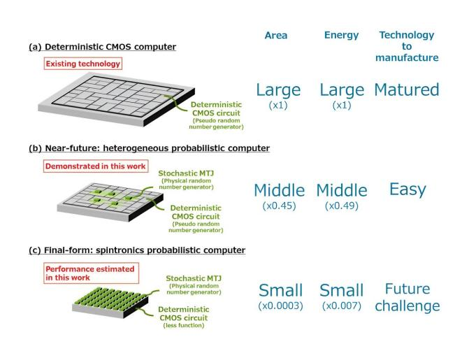
A schematic illustrating the difference in the current deterministic CMOS computer (a), near-future heterogeneous version of the probabilistic computer, and (c) the final form of the probabilistic computer fully based on the spintronics technology. The table on the right side represents the comparison between them in terms of the chip area, energy consumption, and
