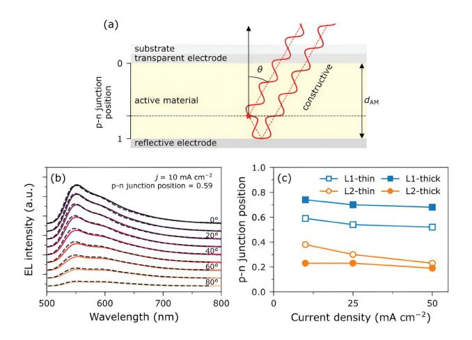
a) Schematic presentation of the optical interference between two light rays that originate from the same spot in the emissive p-n junction (horizontal dotted black line) in a thin-film LEC device, and which are solely distinguished by that one ray is directed directly out of the device through the transparent electrode and substrate, whereas the other ray is directed toward the reflective electrode and first after specular reflection exiting the device. Left part: the p-n junction
