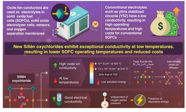
Tokyo Tech researchers demonstrated high conductivity and stability in bismuthcontaining Sillén oxyhalides with triple fluorite-like layers (e.g. 10 mS/cm at 431 °C; 204 times higher conductivity than that of conventional conductors at 310 ° C). Credit: Tokyo Institute of Technology
