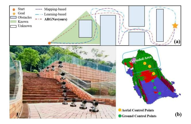
(a) Previous navigation systems had problems predicting occlusions, resulting in higher collision probabilities and suboptimal pathways that consumed more energy. (b) By predicting occlusions in advance, AGRNav can minimize and avoid collisions, resulting in efficient and energy-saving paths. Credit: Wang et al.
