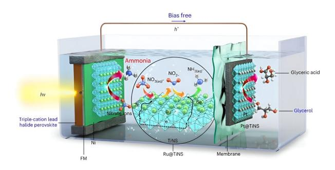
Schematic of the PEC cell used for NH<sub>3</sub> production. Ru@TiNS/Ni/perovskite photocathode is combined with Pt@TiNS anode to achieve a simultaneous biasfree NH<sub>3</sub> production and glycerol valorization. Credit: *Nature Catalysis* (2024). DOI: 10.1038/s41929-024-01133-4
