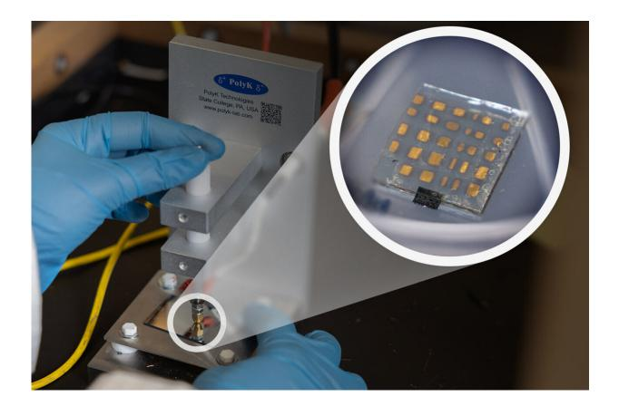
A capacitor prototype with stratified 2D nanofillers embedded in the polymer matrix being tested in a University of Houston lab. Credit: University of Houston
