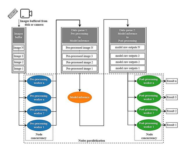
Producer-consumer inference pipeline based on nodes parallelization and
