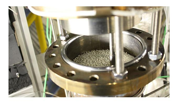
Heat storage system on a laboratory scale: The ceramic beads store the heat. Credit: KALLA, KIT
