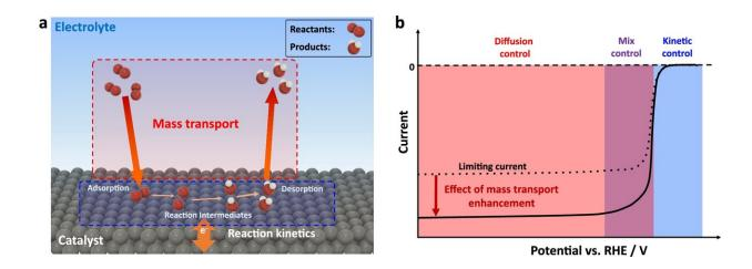
Reaction kinetics and mass transport effects in electrocatalysis. Credit: *Nature Communications* (2024). DOI: 10.1038/s41467-024-46980-8
