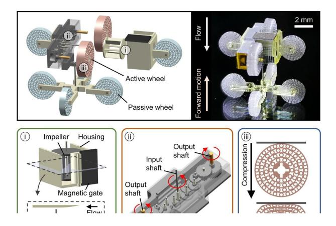
The wireless miniature flow-powered tube robot capable of navigating complex tubular environments. Credit: Chong Hong and Yingdan Wu.
