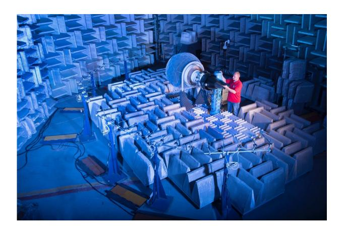
The DGEN380 Aero-Propulsion Research Turbofan (DART) is a small-scale jet engine NASA uses to test new aviation technology. DART is seen here inside its host facility, the Aero-Acoustic Propulsion Laboratory at NASA's Glenn Research Center in Cleveland. This soundproofed chamber ensures researchers can understand the level of noise the engine is producing, as well as keeping the volume low outside. Credit: NASA/Bridget Caswell
