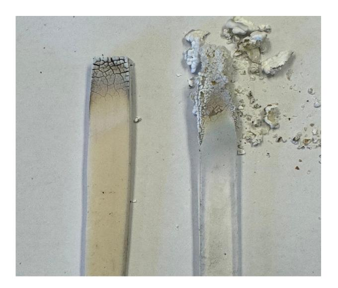
Side-by-side comparison: The team's proposed power pole insulation material (left) next to silicone following a fire-resistance experiment. Credit: RMIT
