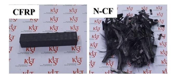
Before and after images of CFRP (Carbon fiber reinforced plastic) recycled into water. Credit: Korea Institute of Science and Technology
