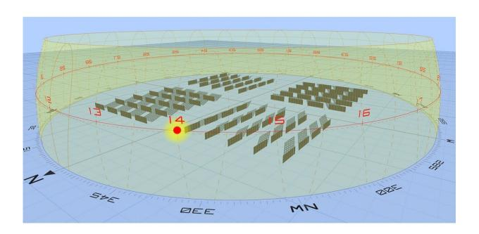
The arrangement of solar panel arrays sketched out in the study. The panels are aligned to catch sunlight along the horizon at virtually any time of day during austral summer. Credit: Argonne National Laboratory and National Renewable Energy Laboratory.)
