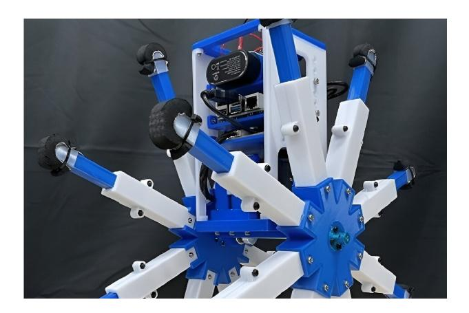
Rimless wheel robot with elastic telescopic-legs. Credit: *Artificial Life and Robotics* (2024). DOI: 10.1007/s10015-024-00943-w
