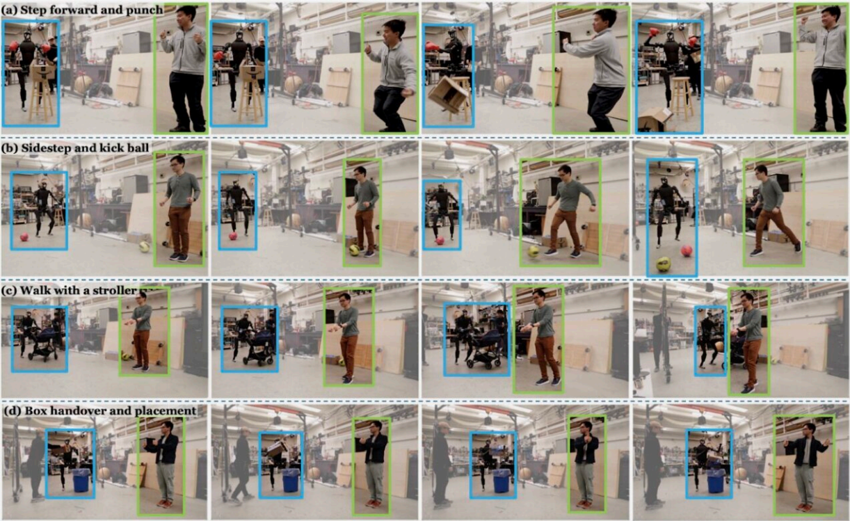
Fig. 1: The humanoid robot is teleoperated in real-time using an RGB camera by the human teleoperator. (a) The humanoid mimics the human teleoperator, advancing one step while delivering a punch to displace a box, followed by a
