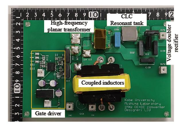
The Kobe University team presented a new circuit design which uses "resonant tank" circuits that can store energy during the switching period and therefore have much lower losses. In addition, they use a component-saving design with flat components printed onto a circuit board, called a "planar transformer," which is very compact and has both good efficiency and thermal performance. Credit: Mishima Tomokazu
