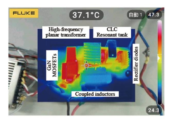
The Kobe University-developed direct current voltage boost converter has much reduced electromagnetic noise and a high energy efficiency of over 91%, which is unprecedented for a MHz drive with high voltage multiplier ratio. This ratio is also more than 1.5 times higher than existing designs. Credit: Mishima Tomokazu
