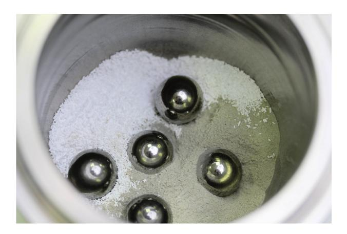
Ball milling chamber contents: spodumene, reactant, and steel balls. Credit: U.S. Department of Energy, Ames National Laboratory
