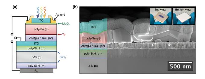
Device architecture of the three-terminal monolithic selenium/silicon tandem solar cell. (a) Schematic illustration of the device structure using either ZnMgO or TiO<sub>2</sub> as the n -type contact. (b) Cross-section SEM image of the tandem solar cell. Photographs of the device are also shown. Credit: *PRX Energy* (2024). DOI: 10.1103/PRXEnergy.3.013013
