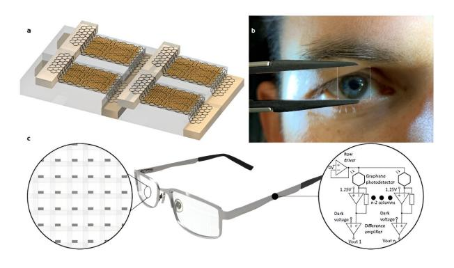
Transparent image sensor concept. a, Digital render of a 2x2 image sensor pattern, showing ITO contact lines (transparent gold), graphene structures (black hexagons), and quantum dots (copper dots). b, 8x8 array on quartz substrate and with ITO contact lines, displayed over an eye. c, Concept of the integration of the transparent image sensor and non-local readout electronics on spectacles. Left inset: schematic representation of the array structure. Dark gray pattern
