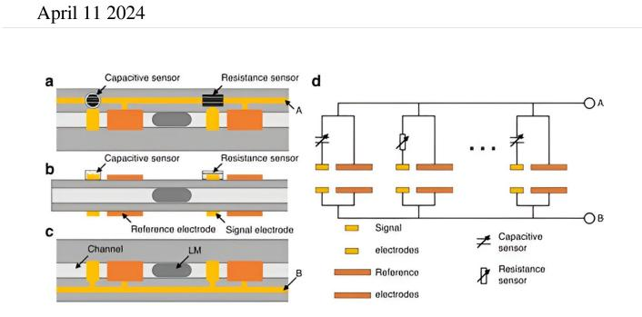
a Schematic top view, b side view, and c bottom view of the switching mechanism. d Equivalent circuit of the SSM. We connected the sensors and signal electrodes to serially arranged electrodes. Credit: *Credit: Microsystems & Nanoengineering* (2024). DOI: 10.1038/s41378-024-00652-1
