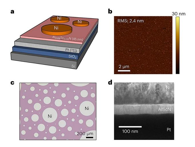
Illustrations of the ferrodiode device. **a**–**d**, A schematic (**a**), AFM height image with root mean square (RMS) roughness (**b**), optical microscopic image of the upper surface (**c**) and cross-sectional TEM image (**d**) of the Ni/Al<sub>0.68</sub>Sc<sub>0.32</sub>N/Pt(111) MIM device. Credit: *Nature Electronics* (2024). DOI:
