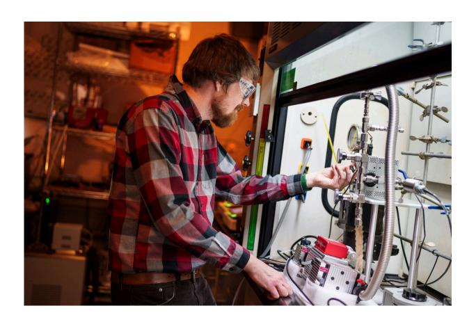
Matthew Paul, a Sandia National Laboratories geosciences engineer, works on a gas adsorption system in a fume hood as part of a project to see if depleted petroleum reservoirs can be used for storing carbon-free hydrogen fuel. Credit: Craig Fritz
