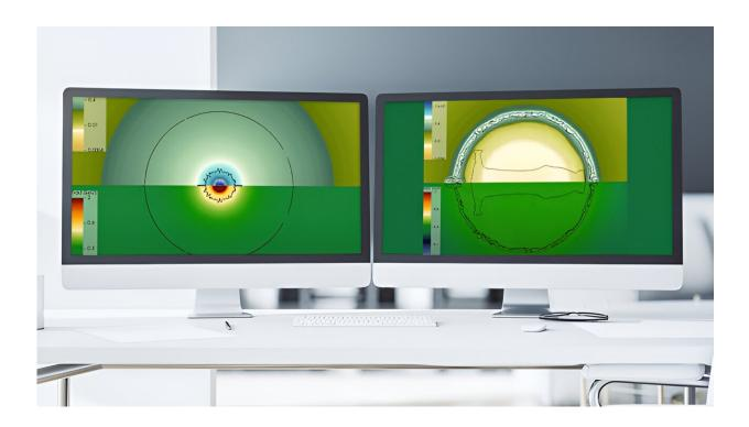
A 2D MARBL simulation of the N210808 "Burning Plasma" shot performed at the National Ignition Facility at the onset of ignition. This calculation consists of 19 million high-order quadrature points and ran on El Capitan predecessor system rzAdams (on AMD MI300A GPUs). Credit: Rob Rieben.
