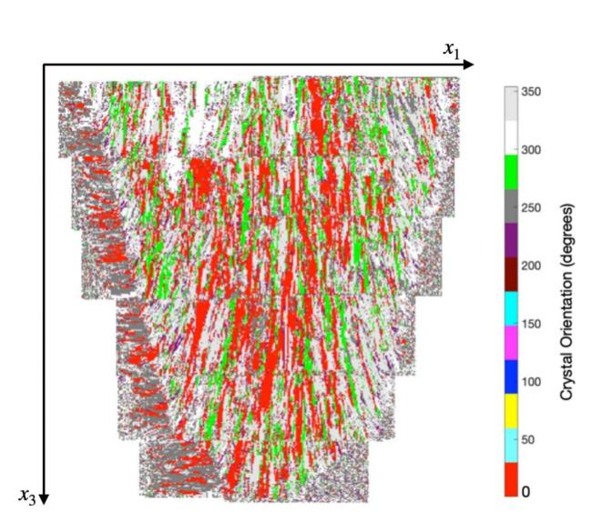
Fanned grain structure of a heterogeneous weld structure. Credit: *Waves in Random and Complex Media* (2024). DOI: 10.1080/17455030.2024.2341283
