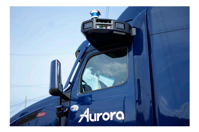
A self-driving tractor trailer is displayed at a test track in Pittsburgh, Thursday, March 14, 2024. The truck, outfitted with 25 laser, radar and camera sensors, is
