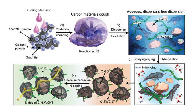
Schematic diagram of SiA/nanocarbon (NC) composite powder preparation process. Credit: *Advanced Functional Materials* (2023). DOI: 10.1002/adfm.202311353
