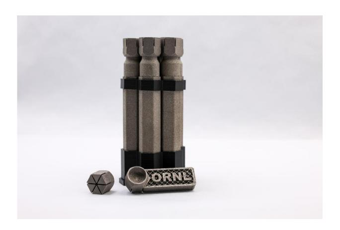
ORNL researchers used electron-beam additive manufacturing to 3D-print the first complex, defect-free tungsten parts with complex geometries. Research was performed at DOE's Manufacturing Demonstration Facility at ORNL. The MDF, supported by DOE's Advanced Materials and Manufacturing Technologies Office, is a nationwide consortium of collaborators working to innovate, inspire and catalyze the transformation of U.S. manufacturing. Credit: Michaela Bluedorn/ORNL, U.S. Dept. of Energy
