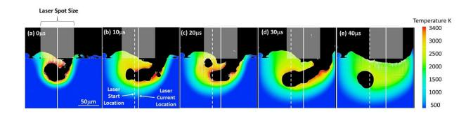
A model view of a keyhole defect forming. The slide that is farthest to the right shows vapor trapped within the cooling metal. APL is aiming to prevent defects like this through development of novel sensing methods that detect the anomalies before they fully form. Credit: Johns Hopkins APL
