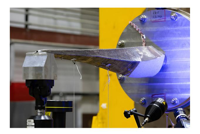
The 3D-printed stainless steel tidal turbine spar undergoes testing at NREL. Credit: Joe DelNero, NREL
