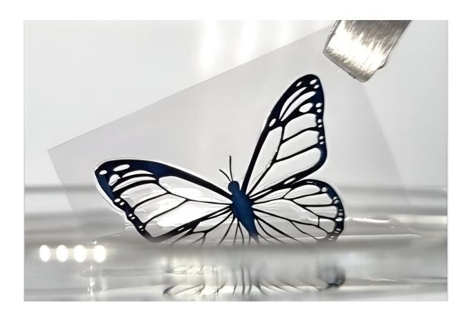
Laser-fabricated conductive hydrogel micropatterns that can strongly adhere to various polymer substrates even after harsh mechanical stimuli. Credit: Daeyeon Won, PhD, SNU
