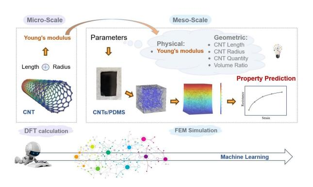
An illustration of the machine learning model framework, showing its application in predicting the electro-mechanical behavior of CNTs/PDMS composites. Credit: Science China Press
