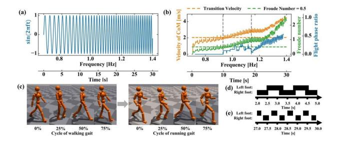
Transition process from walking to running controlled using the AI-CPG method. (a) Sinusoidal signals with increasing frequency were used as input to the rhythm generator of the CPG controller. (b) Center-of-gravity velocity, Froude number and flight phase ratio. The black dashed lines indicate where the gait changes. (c) Transition from walking to running. (d) Time diagram of the
