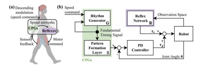
Central pattern generator (CPG) and reflex network coordinated by speed adjustment commands from a higher-level nerve center (a), and overall control framework (b). Credit: Tohoku University
