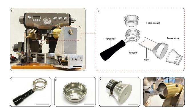
Customized ultrasonic coffee brewing machine. a) Photograph of the machine. b) Schematic of the parts for the ultrasound transmission into the coffee basket. c-f), Photographs of the portafilter (with corresponding window), filter basket, transducer, and the horn, respectively. Credit: *Ultrasonics Sonochemistry* (2024). DOI: 10.1016/j.ultsonch.2024.106885
