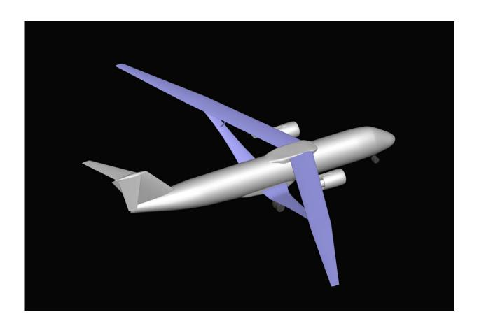
This image of a Transonic Truss Braced Wing airplane represents a digital model created by Aviary, a new computer modelling tool aeronautical engineers can use to innovate new aircraft designs, The Aviary code builds on NASA's decades of experience using highly advanced computer code for aviation. Aviary is a resource created by NASA's Transformational Tools and Technologies project. Credit: NASA
