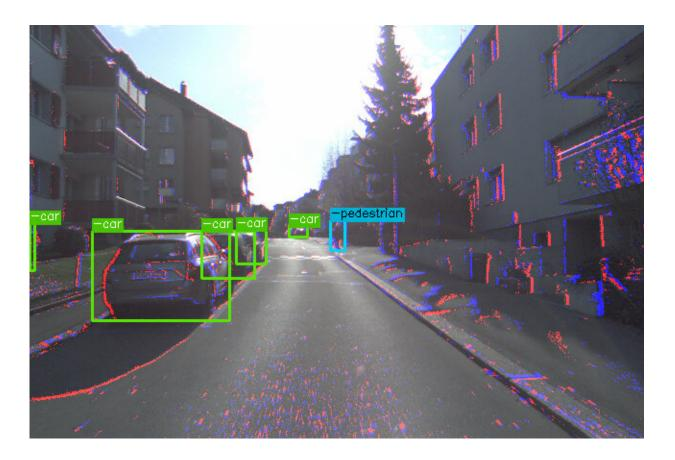
The image shows both color information from the color camera and events (blue and red dots) from the event camera; bounding boxes show the detection of cars by the algorithm. Credit: Robotics and Perception Group, University of Zurich
