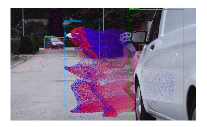
The image shows both color information from the color camera and events (blue and red dots) from the event camera generated by a pedestrian running. Credit: Robotics and Perception Group, University of Zurich
