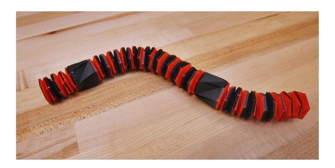
The robot is made of segments that can fold into a flat disk and extend into a cylinder. Partial folds bend the robot and allow for motion and steering. Credit: Frank Wojciechowski/Princeton University
