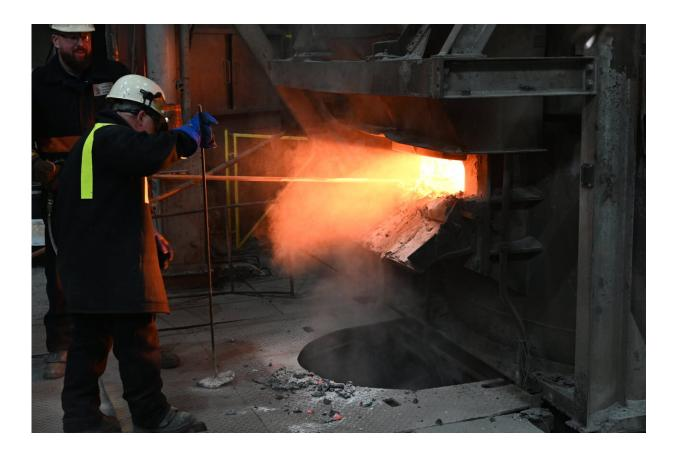
Photographs of the first electric cement production in an electric arc furnace at the Materials Processing Institute, UK. Credit: Materials Processing Institute
