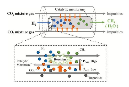
Researchers from Japan and Poland have developed a reactor design that efficiently captures CO<sub>2</sub> emissions and converts them into usable methane fuel. This breakthrough could significantly reduce greenhouse gas emissions, paving the way for a carbon-neutral future. Credit: Professor Mikihiro Nomura SIT, Japan
