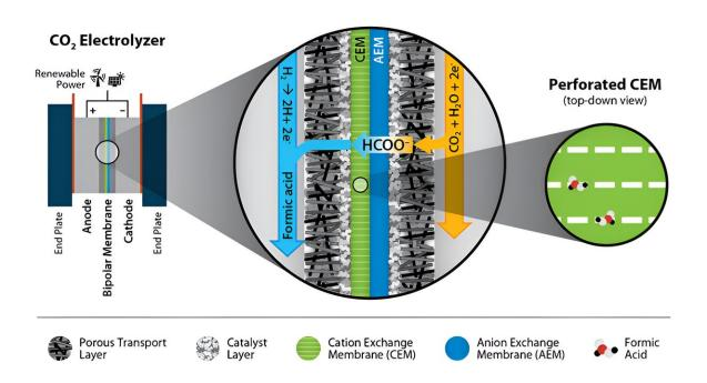
The novel perforated cation exchange membrane (CEM) architecture in a  $CO_2$  electrolyzer to achieve energy efficient and durable formic acid production. Credit: *Nature Communications* (2023). DOI: 10.1038/s41467-023-43409-6
