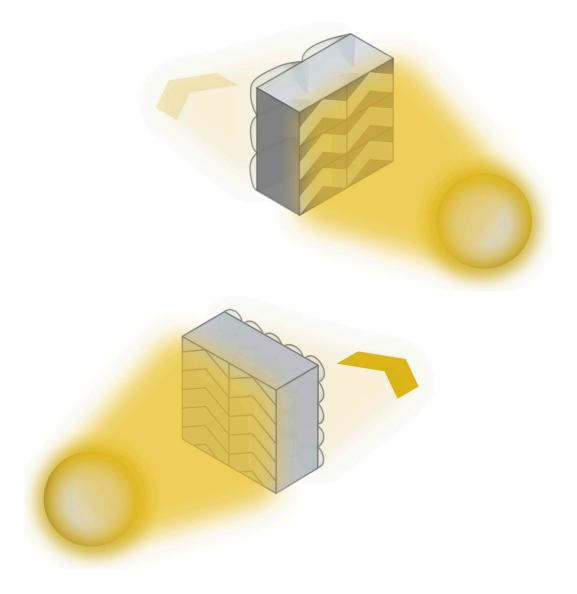
Principle of a conventional micro-optical projector based on apertures (top) and the new projector with irregular lens arrays (bottom). Credit: Fraunhofer IOF
