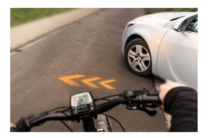
The turn signal is projected onto the road in a dynamic movement and indicates when the car is changing direction. Thanks to the high luminous intensity, the signal is clearly visible even in daylight. Credit: Fraunhofer IOF
